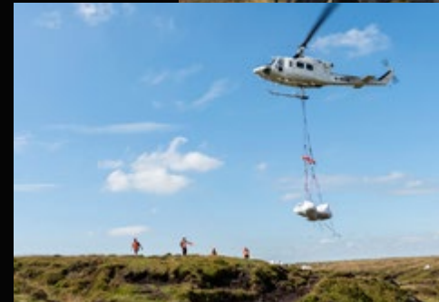
Airlifting bags of Brash for covering dried peat bogs as part of a peatland restoration project at Kinder Scout, Derbyshire
